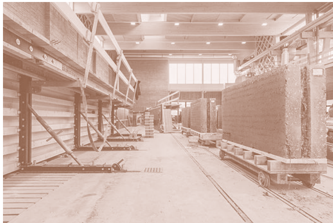
Fig. 19. Manufacturing of large compressed earth blocks at the ERDEN Werkhalle.
