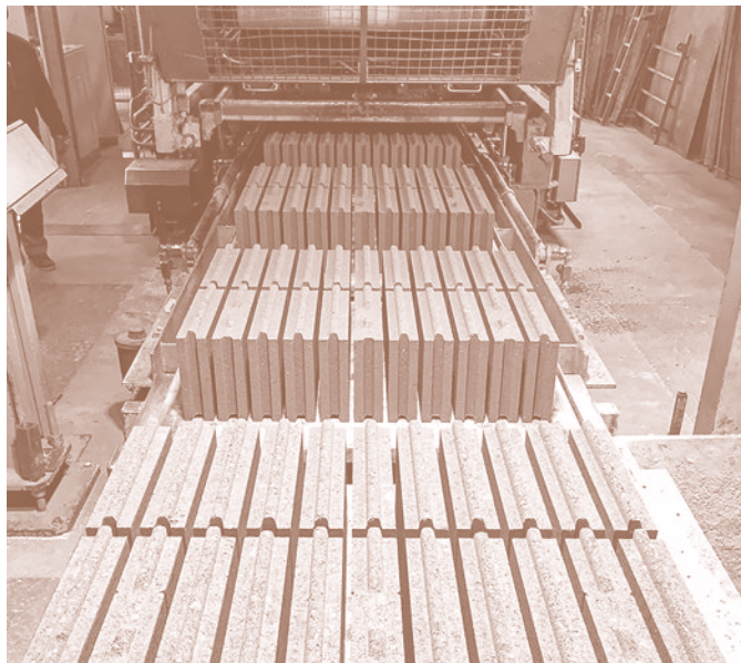
Fig. 25. Manufacturing of the interior partition modules at Terrabloc.
